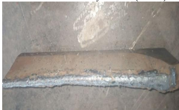
2-rasm. Ishchi yuzasiga PP-NP-T(N), 35V9X3CF markali kukunli sim qoplangan yo'naltiruvchi lineyka
